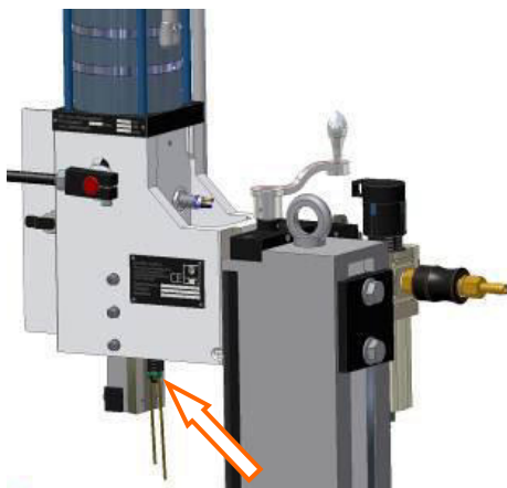
Connect the return spring
